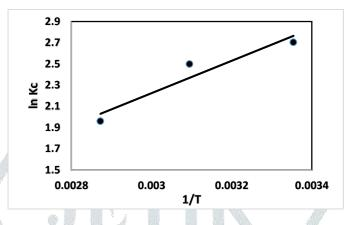
Fig. 8: Plot of ln Kc Vs 1/T for adsorption of Rhodamine B dye on nosean to determine  $\Delta$ H (Enthalpy change) and  $\Delta$ S (entropy change).
