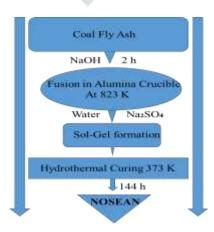
Fig. 2: Flow-sheet for hydrothermal synthesis of nosean using coal fly ash
