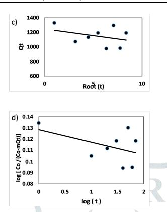
Fig.9: Different kinetic models for adsorption of Rhodamine B dye on nosean at room Temperatures, (a) Pseudo-first order, (b) Pseudo-second order, (c) Intra-particle diffusion model and (d) Bangham's model.
