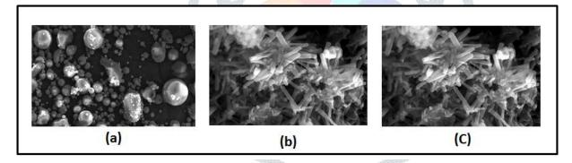
Fig. 4. SEM immages of (a) Coal fly ash, (b) Nosean and (c) Dye adsorbed nosean.
