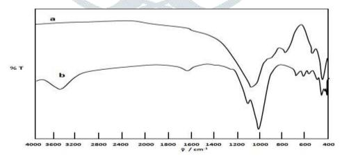
Fig. 2: FT-IR of (a) Coal fly ash and (b) Nosean
