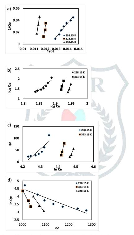
Fig.7: Different adsorption isotherms for adsorption of Rhodamine B dye on nosean at Different temperatures. (a) Langmuir adsorption isotherm, (b) Freundlich adsorption Isotherm, (c) Temkin adsorption Isotherm and (d) Dubinin-Radushkevich.
